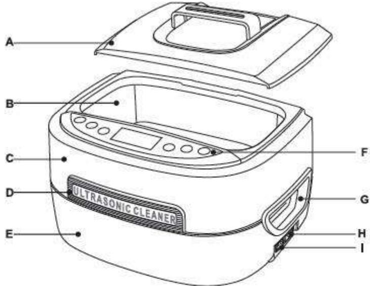
**A.** Top cover      **B.** Stainless steel tank      **C.** Top housing
